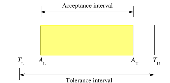
Figure 12 – Binary conformity assessment where decisions are based on measured quantity values. The true value of a measurable property (the measurand) of an item is specified to lie in a tolerance interval defined by limits (T_L, T_U) . The item is accepted as conforming if the measured value of the property lies in an acceptance interval defined by limits (A_L, A_U) , and rejected as non-conforming otherwise.
